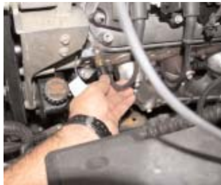
There is a water temp sensor in the front of the driver side head that is used by the engine computer. The 12mm plug located at the rear of the passenger side head can be removed to provide a locating point to install a sending unit for your coolant gauge (Factory, VDO ECT.) The head can be drilled and tapped for a pipe thread or S&P can provide you with a bushing to go from 12mm to either female 1/8, 1/4, 3/8 & 1/2 pipe.
