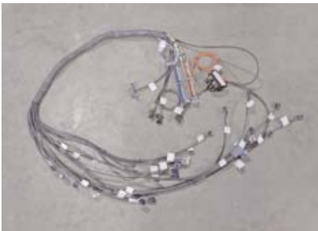
S&P 5.3 engine harness. All connections are labeled for easy connection. The S&P harness comes with instructions and wiring detailed info on wire colors and plugs or can be downloaded for the website. www.hotrodlane.cc
