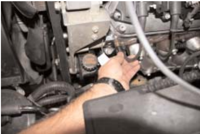
The two prong coolant temp sensor at the front of the driver side head connects to the S&P harness to provide the computer with the engine temp.
