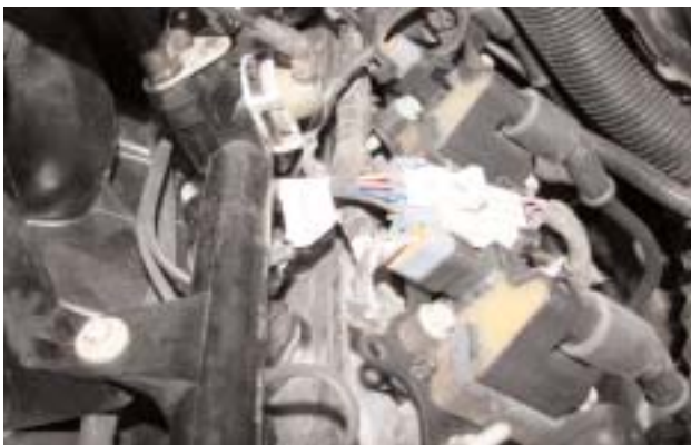
There are two coil plugs (one for driver side and one for the passenger side). These will plug to the center of each coil rack.
