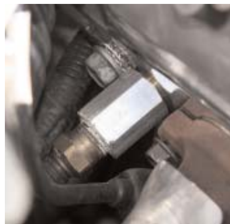
S&P coolant adapter 12mm to 3/8 pipe allowed us to use the Tahoe's original coolant gauge sending unit into the back of the passenger side head.
