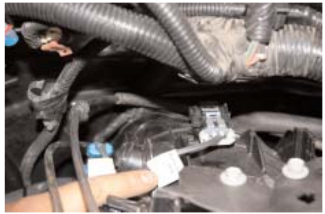
Plug the wire labeled MAP sensor into the map sensor located at the rear of the intake manifold.
