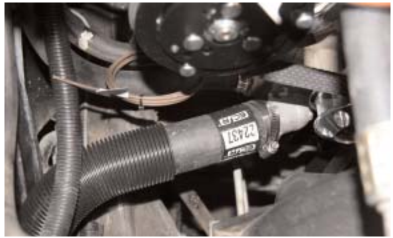
We attached a stock '99 truck lower radiator hose to the lower waterneck and ran it to the lower radiator connection.
