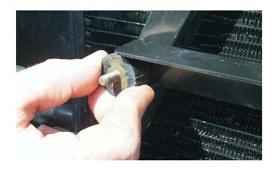
150. Install the heat exchanger onto the studs of the rubber mounts and secure it with the nuts supplied and a 10mm socket wrench.
