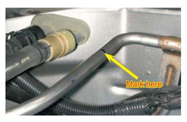
48. Using a tubing cutter, hack saw or cut off wheel, cut the air injection tube in half on the 1 3/4" mark made in step 47. Use a file to remove any sharp edges on the tube.
