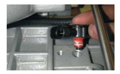
64. Using a 4mm Allen wrench, install the MAP sensor retaining clip with the provided 6mm button head screw as shown.
