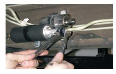
165. Lubricate O-rings and threads of U-bend adapter and install on discharge side of fuel filter. Position as in photo.
