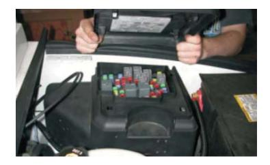
118. Pull back on the two tabs holding the relay centers main cover off.
