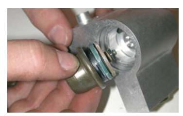
68. Using a pair of C-clip pliers install the new supplied C-clip into the fuel manifold as shown. (Make sure that the clip seats into the machined grove in the manifold.)
