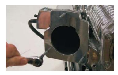
74. Remove the EVAP solenoid from the stock manifold with an 8mm socket wrench.
