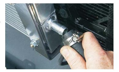
158. From the remaining length of hose, connect one end to the inlet barb of the intercooler reservoir with a #10 clamp.
