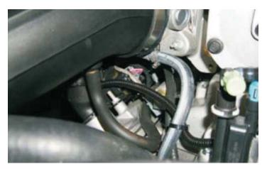
116. Remove fender to firewall brace bracket to gain access to the fuse relay panel, on driver side.
