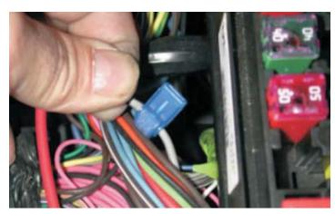
127. Connect the yellow wire from the relay into the T-tap connector installed in the last step.
