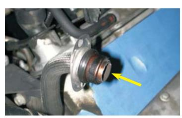
56. Take the new supplied coolant vent pipe and test fit to the front of the cylinder heads. Check for clearance between the pipe and the alternator bracket as shown.
