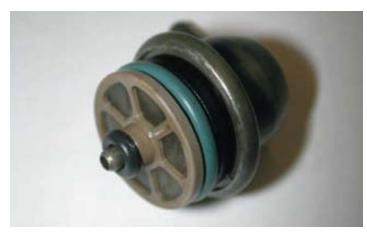
67. Using a small amount of grease or oil lubricate the two O-rings on the fuel pressure regulator and push it into the new supplied fuel manifold as shown.
