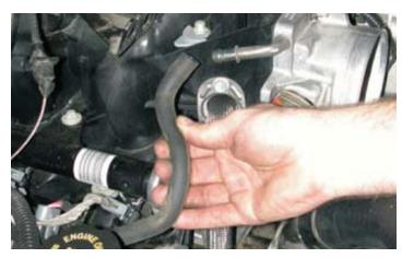
19. Using a 10mm socket wrench remove the 6mm bolt holding the (EGR) tube to the intake manifold. NOTE: Some vehicles may not have a (EGR) system, skip steps 19 and 20.
