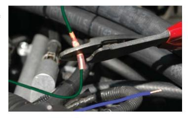
98. Use a heat gun (or hair dryer set on high) to shrink the connectors to the wires. It is not adequate to just crimp the wires together! You MUST shrink the connectors down to seal them from moisture contamination and possible oxidation.
