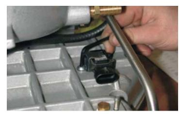
65. Remove the stock fuel pressure regulator from the fuel rail by disconnecting the vacuum hose, pulling off the spring clip and pulling the regulator out. Be careful not to lose any of the small O-rings on the regulator.
