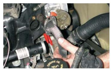
21. Remove the throttle and cruise control cables from the plastic plate on top of the engine. Remove the small plastic clips from the cables. (Skip this step if your vehicle has a fly by wire system, and has no cables.)
