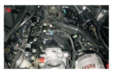
24. Disconnect the eight fuel injector connections by gently pulling up on the gray plastic release trigger on the connector and then pulling firmly on the connector itself.
