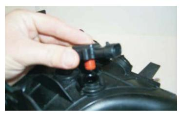
63. Put some lubricant on the MAP sensor seal and press the MAP sensor into the provided hole in the supercharger manifold as shown.
