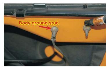
131. Locate the single black ground wire from the relay, strip the insulation back ¼" from the end and then firmly crimp the ring terminal on the end. Install the black wire with its ring terminal on the body ground stud from the previous step and secure it firmly with the original nut.
