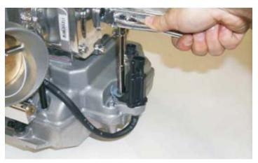
77. Remove factory GM idler with a 15mm socket wrench.
