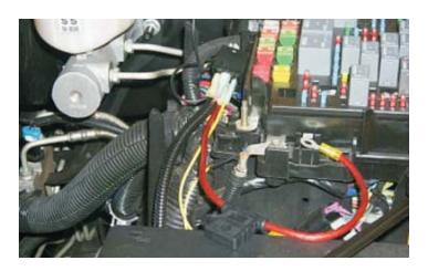
126. In the wiring below the fuse/relay center, locate the gray fuel pump wire that goes from the relay center down the frame towards the rear of the vehicle. Use a 12 volt automotive test light or voltmeter to check that you have the correct wire. With the battery temporarily connected, switch the ignition on and your test light should glow for about 3 seconds and then go out when you have located the correct wire. Install a T-tap connector onto the gray fuel pump wire.
