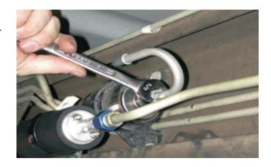
166. Wrap inlet hose & fitting around to filter adapter, and "click" into place.
