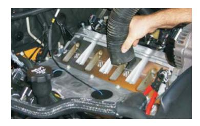
38. Cover the intake ports with tape or clean rags to keep dirt and objects from entering the engine. (Remember, be clean.)
