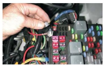
129. Install the positive terminal from the relay to the positive lug as shown. (This is the wire with the fuse holder in it.)
