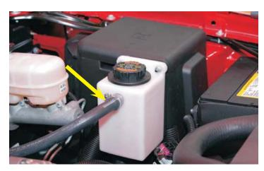
159. Cut the remaining end of the hose to length and connect it to the "T" connection on the supercharger with a #10 clamp.
