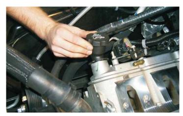
83. Spray silicone or some mild soap and water solution on cylinder head surface to lubricate. This makes the intake manifold slide around a little to help line up the holes. (Do not use anything that will damage the intake gaskets such as petroleum based products, etc.)
