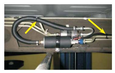
168. Cut the pump wiring loom installed earlier in step 126 so that the black and red wires will reach the new pump.
