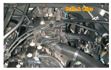
23. Disconnect the following electrical connectors. Eight fuel injectors, Manifold absolute pressure sensor (MAP), Evaporative emission canister purge solenoid (EVAP), Alternator and Knock sensor.
