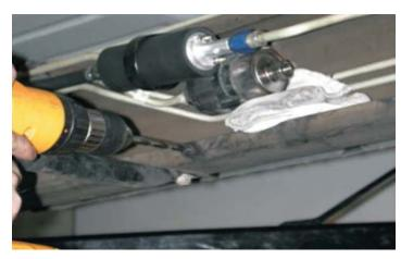
164. While supporting the pump using back-up 7/8" wrench, tighten fuel line fittings. (Make sure adapter does not get loosened.)
