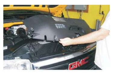
145. Remove the grille assembly by first removing the upper retaining bolt with a 10mm socket wrench.
