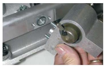
71. Using the small 3/16" hose supplied, connect one end to the small barb on the pressure regulator. Connect the remaining end of the hose to the barb at the left rear of the supercharger manifold.
