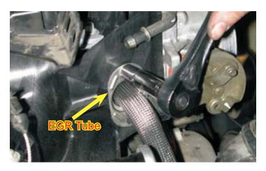
20. Grab the (EGR) tube and pull it out of the intake manifold as shown. Make sure you have the rubber O-ring out of the manifold.
