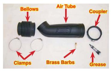
111. Assemble the bellows and coupler to the air tube. **NOTE:** The position of the clamp screws. The screws must be facing up so that you can install the assembly on the vehicle.
