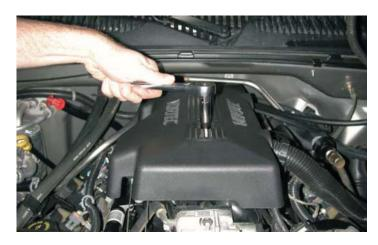
8. Lift plastic shield from top of engine.
