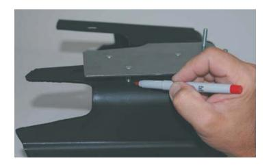
122. Place the reservoir bracket in location on the holes. Secure the bracket on the inside of the cover with the three nuts supplied. Tighten the nuts with a 10mm socket wrench.
