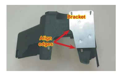
121. Mark the location of the three mounting studs on the cover and then drill 1/4" holes in these locations.
