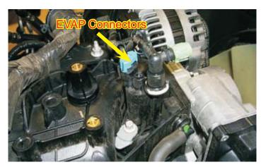
29. Lift the electrical harness from the top of the engine and set off to the side.
