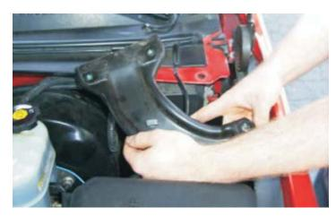
117. Firmly grasp the relay centers cover and lift off.
