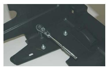
123. Assemble the components of the intercooler reservoir/pump assembly as shown in this picture. **NOTE: The hose and electrical connections and orient the pump as illustrated.**
