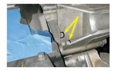
58. Using a file or die grinder, remove material from the alternator mounting bracket marked in the previous step. Once clearance is achieved, recheck with the new vent pipe. Ensure that the vent pipe does not touch the alternator bracket.
