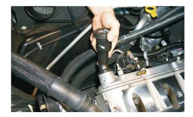
82. Install the short oil filler neck supplied by inserting it into the valve cover and rotating it 180 degrees clock-wise. Transfer the oil fill cap from the long neck to the new short one.
