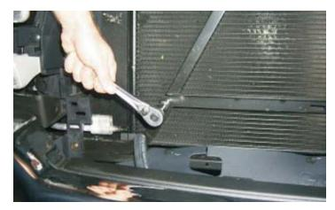
149. Replace the cross member bolts with the rubber mounts supplied. Tighten the mounts securely by hand only.
