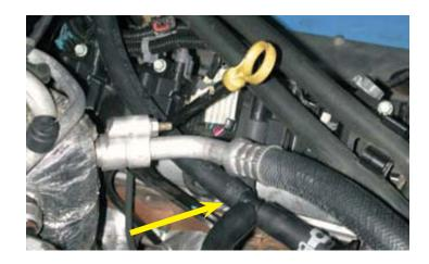
54. If your vehicle does not have EGR system skip steps 54-55. Cut the end of the (EGR) tube off with a cut-off wheel or hack saw. Make sure not to damage the O-ring seal.
