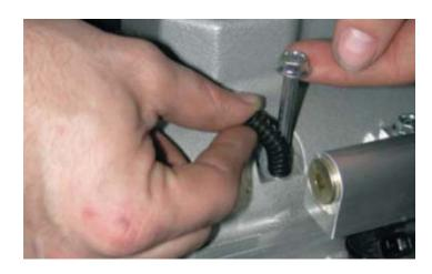
86. Torque all ten bolts gradually and evenly to a torque of 106 in-lbs, using a center-out, crisscross pattern.
