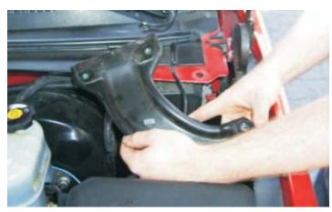
137. Here is the intercooler and its mounting components.
