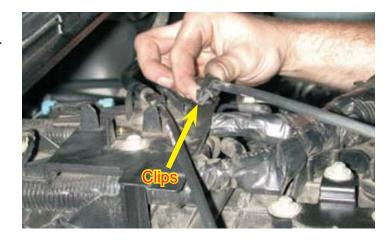
22. Open the large electrical harness retainer clip, then using a 10mm socket wrench remove the bolts holding the plastic wire harness retainer to the intake manifold.
