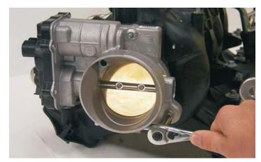
73. Install the three studs removed in the previous step into the new supercharger inlet manifold using a #5 internal Torx socket and wrench.
