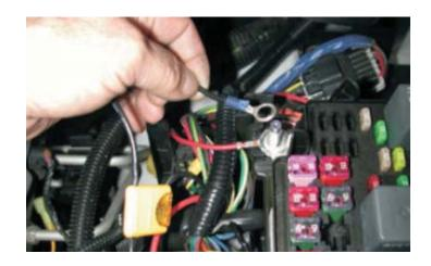
130. Using a 10mm socket wrench, remove the nut from the body ground stud on the firewall as shown.
