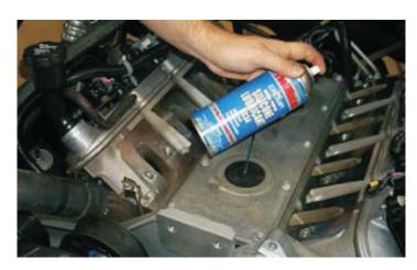
84. Using an assistant, carefully lower manifold assembly into place, being careful not to damage gaskets.
