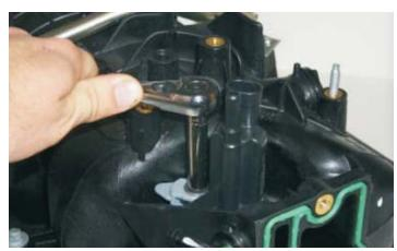
75. Lubricate the O-ring with the supplied grease and press the EVAP solenoid into the hole on the new supercharger intake manifold.
