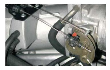
92. If your vehicle is EGR equipped (see steps 54 & 55), remove the 3/8" NPT plug and thread on the EGR relocation manifold. Feed the EGR tube to this manifold, re-use seal and fasten using OE hardware.
