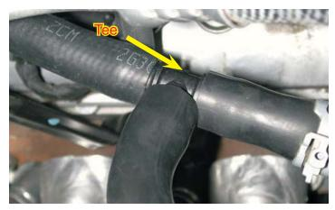
53. Route the modified air injection hose assembly as show in the above picture.
