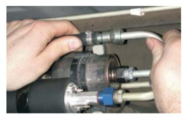
167. Use tie wraps supplied in kit to fasten hose & wires out of harm's way, and to allow smooth bends.
