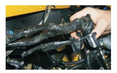
94. Route the wiring harness over the left side fuel rail and attach it to the supercharger manifold as shown, using the Adel clamp and bolt supplied.
