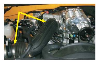
115. Attach the PCV hose from the right (passenger) side valve cover to the brass barb on the bottom of the air tube. Connect the PCV hose from step 60 to the remaining barb next to the power brake hose connection on the back of the inlet manifold. Connect the power brake hose to the control valve shown in step 33.
