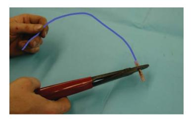
97. Using the color coded wires provided in the 31-12-00-007addendum kit, strip off 3/8" off of the ends of all the wires. Match the color coded wires to the matching wires on the removed plugs, as well as the harness ends, and crimp on the wires with the provided crimp/shrink connectors.
