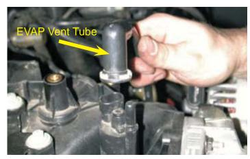
31. Remove the positive crankcase vacuum hose (PCV) from the intake manifold on driver side.
