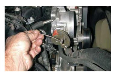
16. Using a pair of pliers, squeeze the plastic retainers on the throttle and cruise cables, and remove from the bracket.
