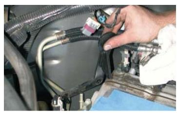
41. Using a 10mm socket wrench, remove the two or four coolant vent pipe bolts. (Some models have a small pipe in the front and some have a large pipe that goes from the front to the back.)
