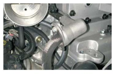
93. Remove the wiring harness from the original bracket.
