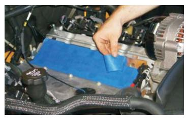
39. Remove the small plastic clips from the knock sensor electrical harness. The intake manifold will not clear if this step is missed.
