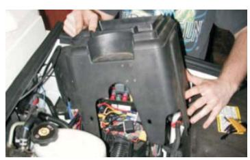
120. Position the intercooler reservoir bracket on the engine side face of the main cover. Align the cut-away of the cover with the edge of the bracket
