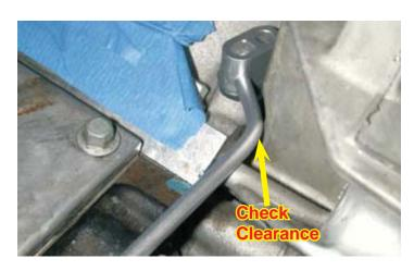
57. Use a felt tip marker and mark the alternator bracket were the coolant vent pipe hits as shown.
