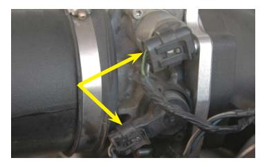
26. At the rear of the of the intake manifold disconnect the Manifold Absolute Pressure (MAP) sensor connector by gently raising the gray plastic retaining clip and then pull the connector free.
