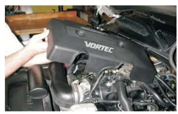
9. Using an 8mm nut driver loosen the two large hose clamps holding the air cleaner duct assembly.
