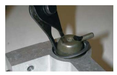
69. Apply a small amount of grease to the new supplied fuel manifold O-ring and set in the machined recessed area on the new driver side fuel rail as shown.
