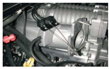
91. Install both cruise control and throttle cables & PCV hose. Check for smooth cable operation.
