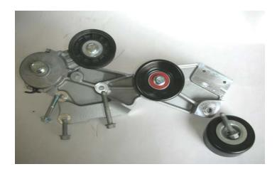
80. In the original tensioner location, install the new tensioner support bracket. Torque all mounting fasteners to 40 ft-lbs. NOTE: The tensioner will come pre-installed on our new bracket. The tensioner was removed for photo clarity in this picture.
