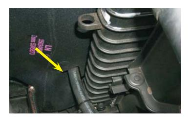
156. Continue the hose to the upper barb on the top of the heat exchanger. At this point cut the hose and push it on the barb. Secure it with a #10 clamp.
