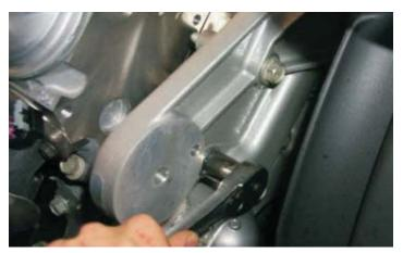
81. Remove the long oil-filler neck from the valve cover by rotating it 180 degrees counter clockwise and pulling it out.
