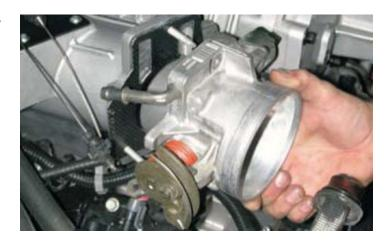
90. Fasten throttle cable bracket and install both cables.
