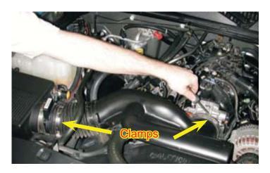
10. Remove the duct assembly by lifting it out. Sight shield and duct assembly will not be reused.
