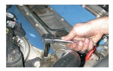
42. Remove the vent pipe assembly. (Make sure that the O-ring gaskets did not stick to the cylinder heads, if so remove them.)
