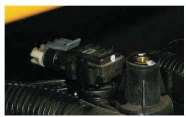
27. Disconnect the engine knock sensor connector and steel-mounting clip from the intake manifold by prying it free with a small screwdriver. Next gently raise the black plastic retaining clip and then pull free the connector from the harness.
