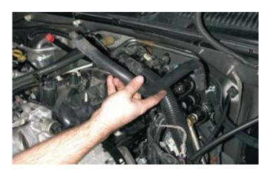
32. Disconnect the small vacuum hose from the rear passenger side of the intake manifold, if so equipped.
