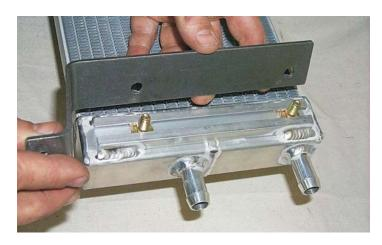
140. Torque the mounting nuts to 18 ft-lbs.
