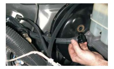
34. With the fuel line disconnect tool supplied, remove the fuel lines from the fuel rails. Caution! The system may be under pressure. Avoid open flame or other sources of ignition.
