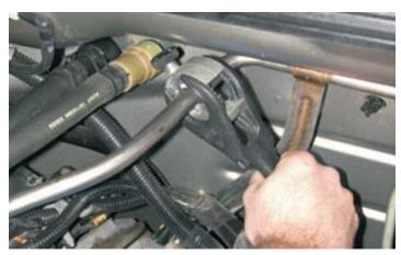
49. Disconnect the two air injection hoses from the other end of the tube and save the factory hose clamp for a later step.
