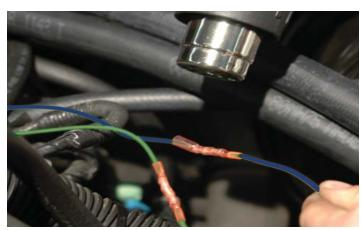
99. When done, use the provided split loom to cover over the extended plugs, some electrical tape at the junction to the old harness and at the plug ends, connect the plugs to the throttle body from whence they were removed earlier.
