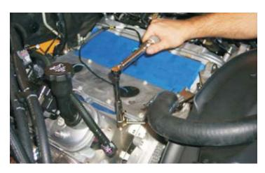
60. Using the new supplied 16" x 3/8" PCV vacuum hose, connect one end to the PCV valve as shown and lay the other end of the hose off to the driver side, out of the way. (To be connected in a later step.)
