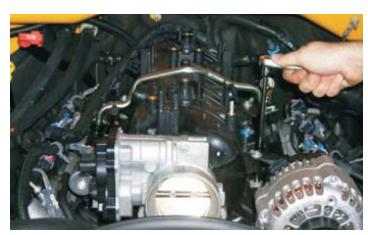
36. Carefully remove the intake manifold assembly and set aside.
