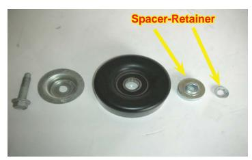
79. Here is the new tensioner support bracket and hardware. The new bracket will locate in the original tensioner location. NOTE: The different fasteners and their locations. Install the 90mm idler and spacer on the idler support bracket. Torque the mounting bolt to 40 ft-lbs.
