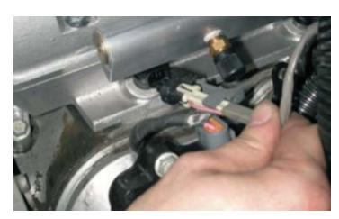
96. For late model vehicles, you must extend the Throttle Position Sensor (TPS), and Idle Air Control (IAC) plugs, by first pulling back the factory Split Loom from the plugs. Cut the wires in a staggered pattern, each wire 1" shorter than the adjacent wire. This keeps the wires from having all connectors in one place. Strip off 3/8" of the insulation from each cut end, and crimp on a provided crimp/shrink connector as shown in this generic picture.
