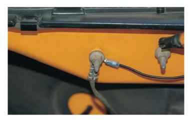
132. Install the intercooler electrical connector into the bottom of the coolant pump. Secure the wiring as necessary with the Tie-wrap straps supplied.
