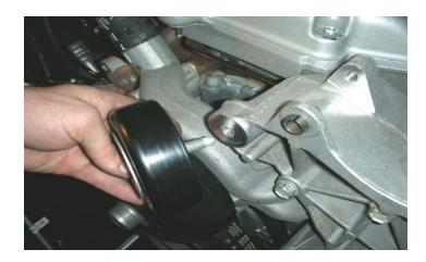
78. Using a soft hammer, knock the factory bolt loose from the idler pulley. The bolt retainer and spacer will not be re-used. **NOTE: The bolt, dust cover and idler will mount to new tensioner bracket.**
