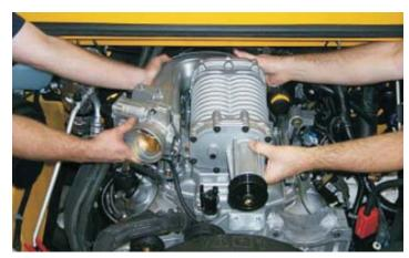
85. Remove the ten spilt looms that support the fasteners. Start all ten bolts by hand.
