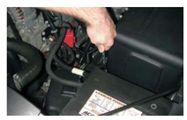
5. With a cool engine remove the radiator cap. (Be careful not to remove the cap if the engine is still hot.)
