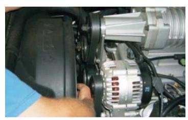
107. Using a screwdriver, remove the four screws that secure the top cover to the base of the air box assembly.
