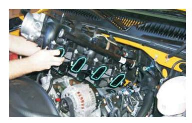
37. Using a vacuum cleaner, remove any dirt or debris from the intake port area. (Be careful not to get any dirt in the intake ports.)
