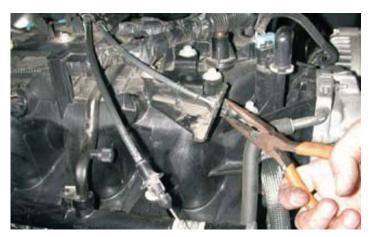
17. Using a long pair of pliers, remove the coolant hoses from the bottom of the throttle body.
