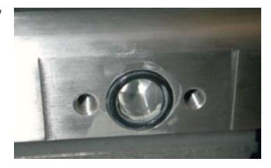
70. Install the assembled fuel manifold to the driver side fuel rail using the two new supplied 6mm bolts. Using a 10mm socket wrench torque the bolts to 106 in-lbs. (Be careful not to pinch the O-ring.)
