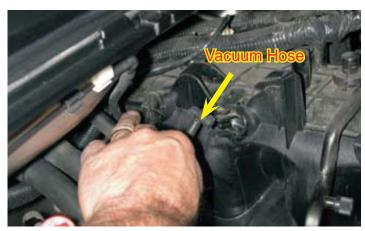
33. Remove the power brake booster hose from the booster by pulling out on the check valve. (Some vehicles have hydraulic assist brakes and do not have this hose.)
