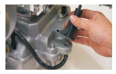
76. Secure the EVAP solenoid on the front of the intake manifold with the OEM mounting bolt using an 8mm socket wrench.
