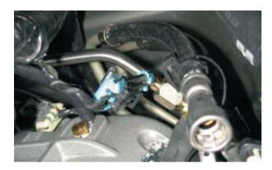
88. Push the fuel line connector on to the fuel manifold. Ensure that the fuel line is pushed all the way on. Pull on the connector to check that it is secure, you should not be able to remove the connector unless you use the removal tool.
