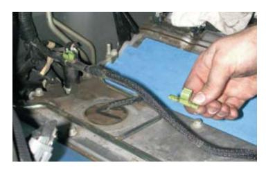
40. Using a 15mm wrench, remove the steel bracket from the rear of the driver side cylinder head. This will not be reused.
