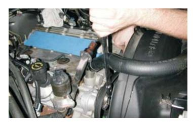
44. Using a 15mm socket wrench or wrench remove the three bolts holding the factory belt tensioner to the bracket and remove the tensioner.
