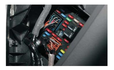
177. Remove the cover from the "Exterior Fuse Panel" located under the hood on the drivers (left) side. Remove the six fuses labeled SEO B1, SEO IGN, INFO, SEO B2, RADIO and RADIO AMP. Download the SuperChips FlashPaq file following the instructions that came with the SuperChips tuner.
