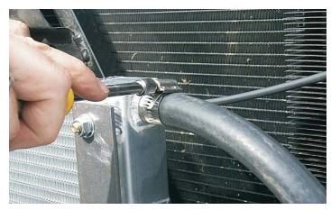
157. From the remaining length of hose, attach one end to the lower barb of the heat exchanger. Route the hose through the slot in the weather shield and on to the outlet barb out the intercooler pump. Cut the hose and secure both ends with #10 clamps.
