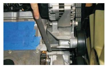
59. Using the stock bolts removed in step 41 install the new coolant vent pipe supplied. Ensure that the O-ring seals are installed correctly. Torque the bolts with a torque wrench and 10mm socket to 106 in-lbs.
