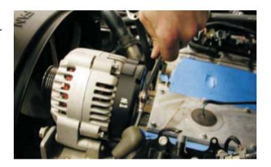
46. With a 15mm socket wrench remove the two bolts holding the alternator to the alternator bracket. Remove the alternator.
