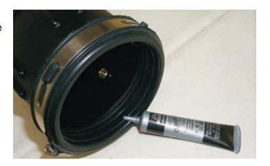
114. Push the bellows end of the air tube assembly on to the air box first, and then install the remaining end with the coupler on to the throttle body. Tighten all clamp screws securely.
