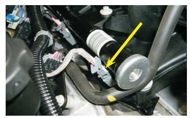
25. On late model vehicles, disconnect the Idle Air Control (IAC) and Throttle Position Sensor (TPS) connectors from the throttle body by releasing the locking tabs first, then squeeze and pull the connectors free. These connectors will need to be extended later.
