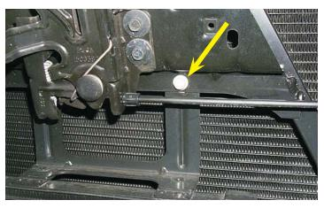
152. Install the upper mounting clamp onto the heat exchanger core using the bolt removed in the previous step. Tighten the bolt securely.
