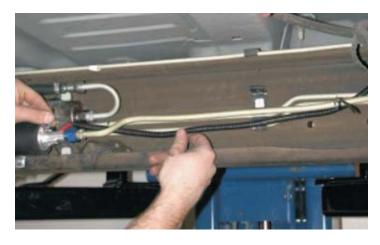
169. The fuel pump wiring must be hooked up correctly to work, the red Positive wire goes to the "+" post on the pump and the black negative wire goes to the "-" post on the pump. (Double check your installation before moving on.)
