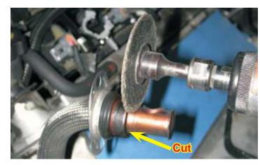
55. File any sharp edges from (EGR) pipe. When finished the (EGR) pipe should look like this.
