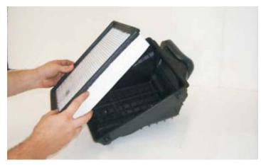
109. Install K&N air filter components and reassemble the air box assembly. Reinstall the completed unit on the vehicle.
