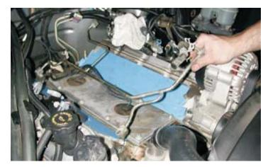
43. Using a 15mm tensioner wrench or breaker bar, remove the stock serpentine belt from the vehicle. The belt will not be reused.
