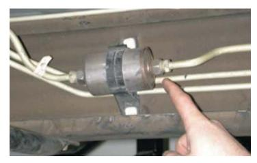
161. Using 5/8" and 13/16" wrenches, disconnect fuel line from filter. Use rags to soak up and fuel. (Be sure to dispose of rags properly.) Do not lose small O-ring on fitting.
