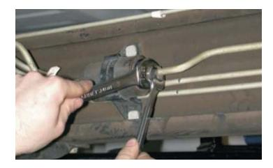
162. Use a small amount of grease to lubricate the O-ring threads of the OE fitting. Carefully bend the tube to run parallel to frame rail and direct into pump discharge fitting.
