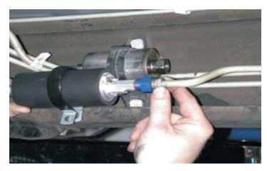
163. Using 21/64" drill carefully drill through bottom of frame rail. Clean up chips, deburr the hole and fasten pump with supplied hardware.
