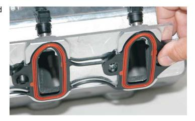
62. Remove the stock MAP sensor from the stock intake manifold by pulling back on the two tabs and lifting the sensor out. Ensure that the orange MAP sensor seal is not damaged, as it will be used.
