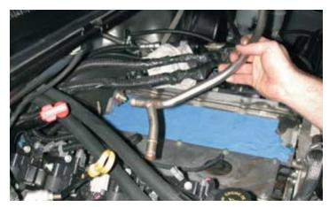
51. Using the new supplied 90 degree 5/8 molded hose cut 2" off the short end and cut 3" off the long end of the hose. Using the factory hose clamp removed in step 49, install the short end of the hose to the air injection tube as show in the picture above.
