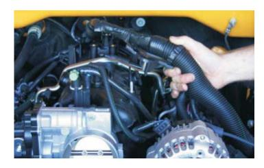
30. Disconnect the (EVAP) vent tube from the solenoid by squeezing the retainer, and then release the tube from the solenoid. Follow the same procedure on the other end of the (EVAP) vent tube and remove the tube from the vehicle.
